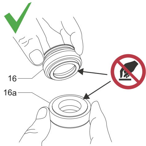
Fig. 19 How to correctly hold the shaft seal
