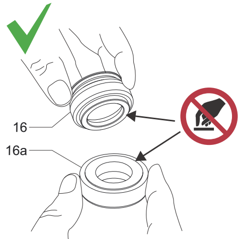
Fig. 15 How to correctly hold the shaft seal
