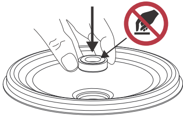
Fig. 21 Fitting the stationary part of the shaft seal
