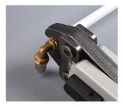
To press the fittings, use a jaw of the same size of the fitting and profile complying with table "Tongs profiles" on page 2:
