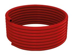
R996T-5 pipes in PEX-b (polyethylene crosslinked with the silane method - crosslinking degree > 65 %) can be used for the water distribution into heating and/or cooling systems. R996T-5 pipes are extruded, in compliance with EN ISO 21003 Standards, with an intermediate (within the thickness of the pipe) anti-oxygen barrier in EVOH, to avoid any type of damage on site and therefore the modest oxygen quantity that permeates from outside towards the inside of the pipe, becomes quite negligible.
