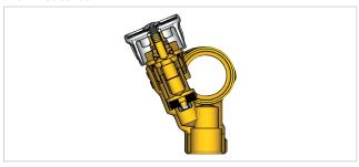
The manifolds are produced using a moulded body, which gives them a combination of extreme solidity and reduced roughness, obtained by machining to remove burrs on all interior surfaces. When looking at a cross-section of the R585C manifold, it is evident that the connecting sections have been designed to obtain the widest passage possible.
